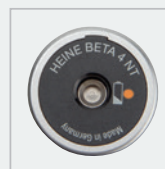
Charge status indicator in the bottom insert
