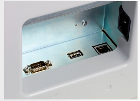
Extended connectivity USB host for inputting patient info by keyboard/barcode reader. LAN and RS-232C for connection to network. XML file output via LAN.
